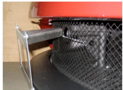
(with the front face vertical) so the slot in the tongue straddles the edge of the triangular vertical sheet metal piece that supports the tow-hook mounting tube from underneath. If the slot fits the sheet metal piece too tightly to slide on this way, then instead you can slide the tongue onto the sheet metal piece as you slide in the bracket. The purpose of this tongue is to keep the bracket from rotating around the mounting bolt due to vibration.
