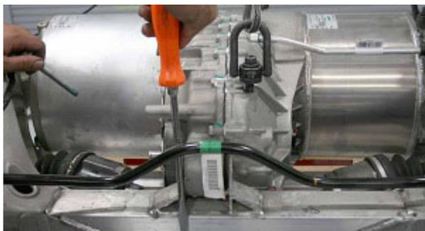
12. Carefully lift the drive unit assembly, making sure to clear the rear of the subframe.
