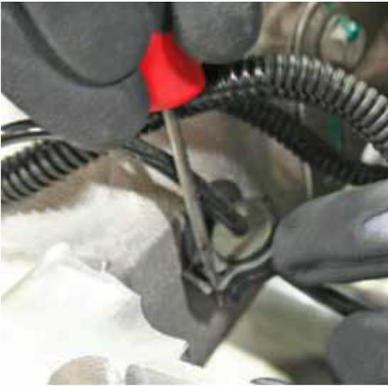
4. On both sides of the subframe, release the bolt that secures the upper link to the knuckle (torque 140 Nm).
