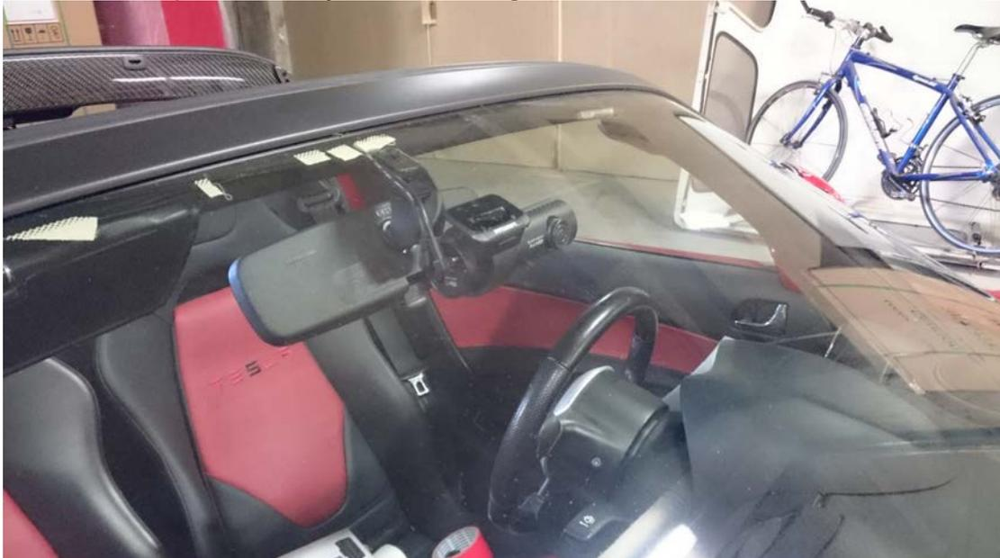
Use the silicone gun to glue the cables to the edge of the window. If you miss some parts or make a mess....use the industrial ethanol with a paper tissue to clean it.
