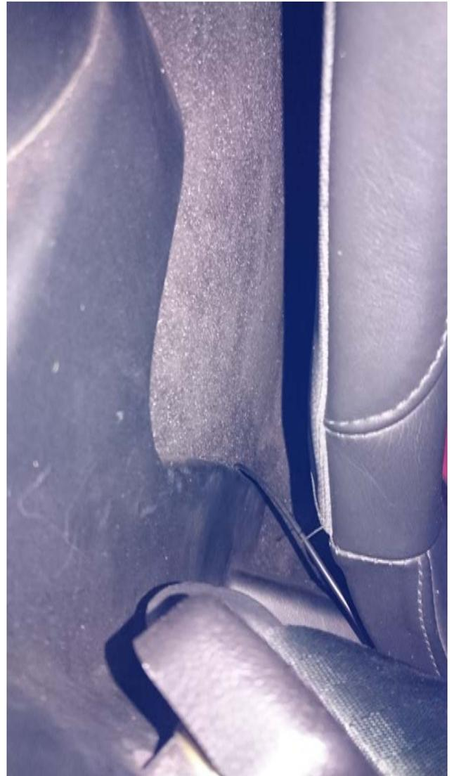
Run the cable under the speaker plastic cover.
