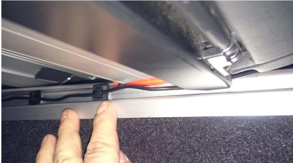
Run the cable through the gap and fish it out inside the fuse compartment.
