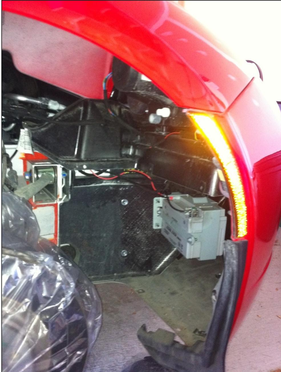
2. There is a much easier way to do this. On the right side of your vehicle on the passenger side, there is a compartment for your fuses. Inside the fusebox we are going to **tap into fuse #13**. It's a 7,5A fuse used for the alarm of your car.
