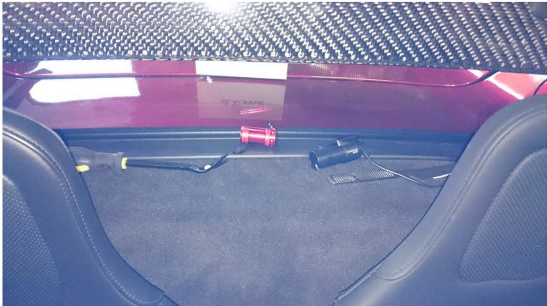
Continue to tuck the signal cable under the plastic cover. You might need to go twice with the cable back and forward because of the length of the cable. Continue the to towards the other speaker.
