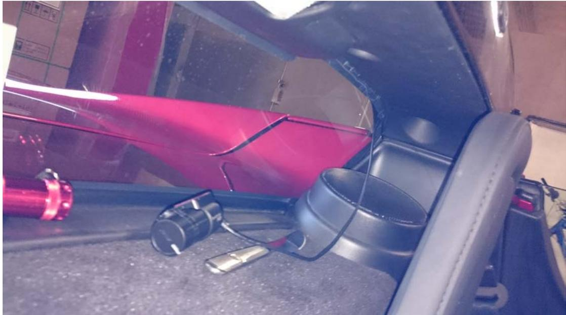
Push the cable and hide it the gaps. It will fall in place. Use the butter knife to tuck it along the window and the plastic on top.
