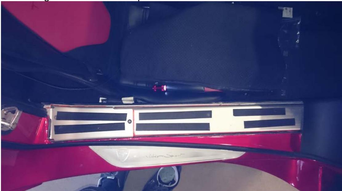
Run the signal cable along side of the side cover. Just open the carpet and push it in.
