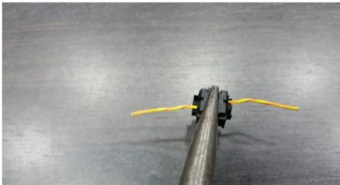
It is essential to secure the adapter with pliers.
