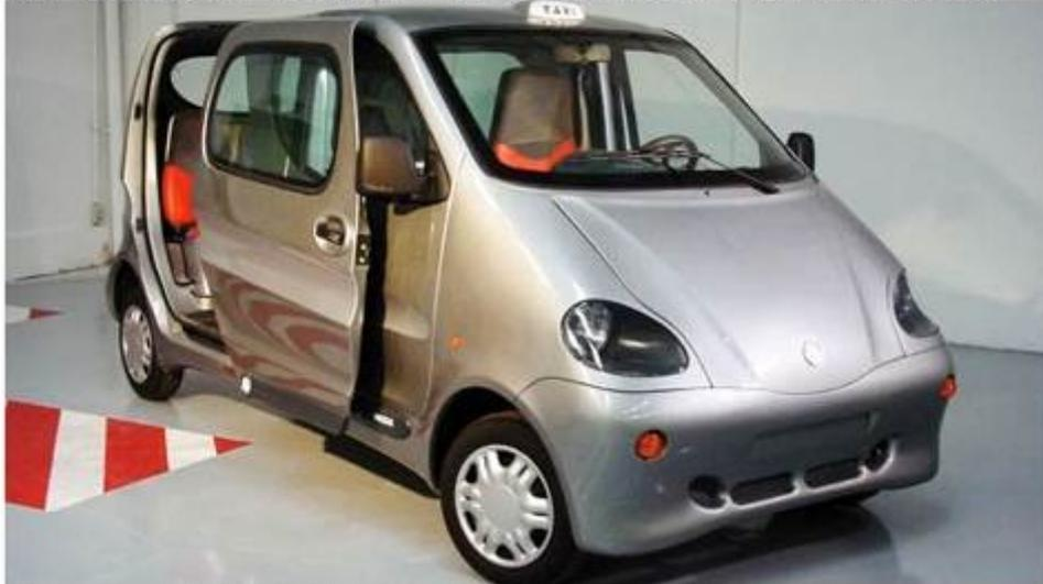
This six-seater taxi, which should be available in India next year, is powered entirely by a tank filled with compressed air.
